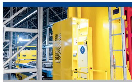
Another lane with 1330 storage spaces is reserved for the storage of (steel) cassettes with the dimensions 3,750x1,200x600/1,200/1,800/2,400 (LxBxH). These are above all intended for interim storage of large products. In order to be able to safely load and transport the cassettes together with their additional load of up to 900 kg, the designers fitted the stacker cranes with specially designed load-handling attachments. The performance of the device is 85 double cycles an hour.
